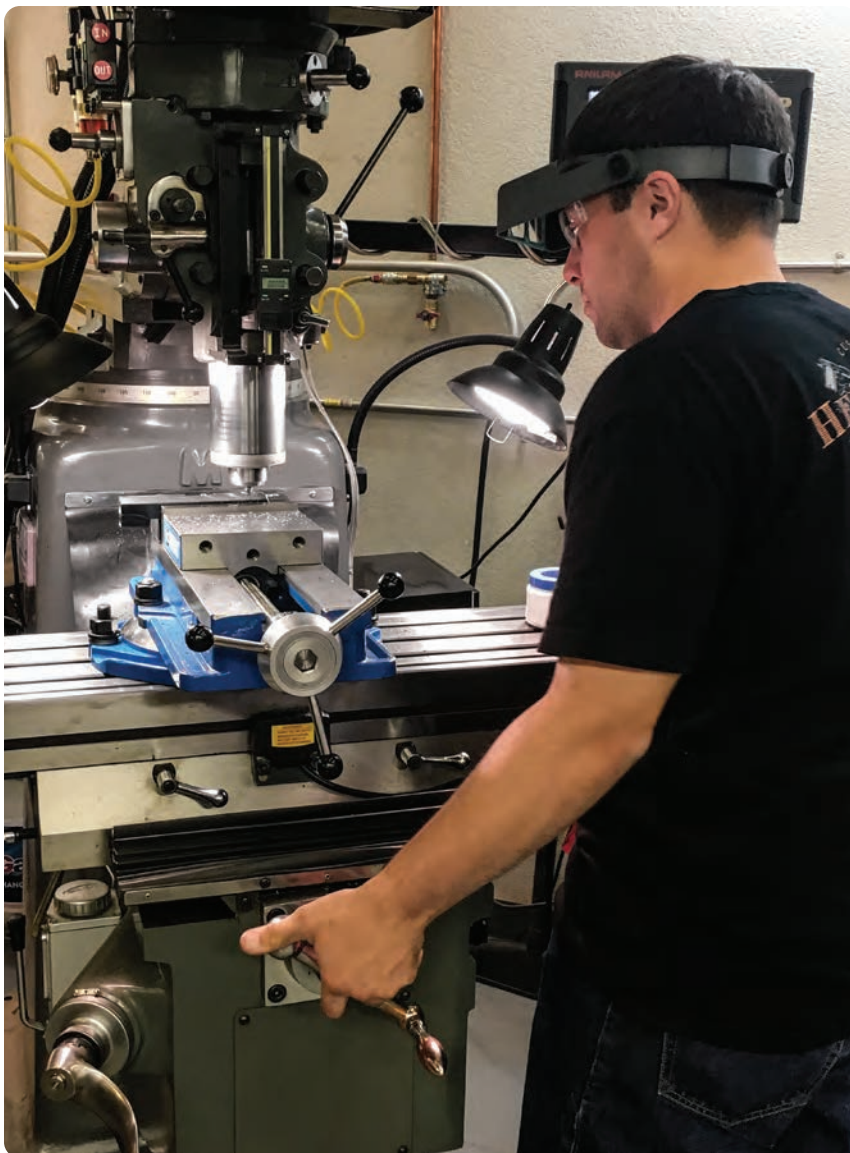
Burton in the Heirloom Precision workshop, machining sight dovetails into a slide.
